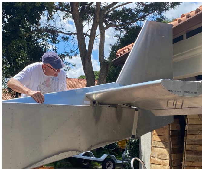
Ant busy on empennage fitting
