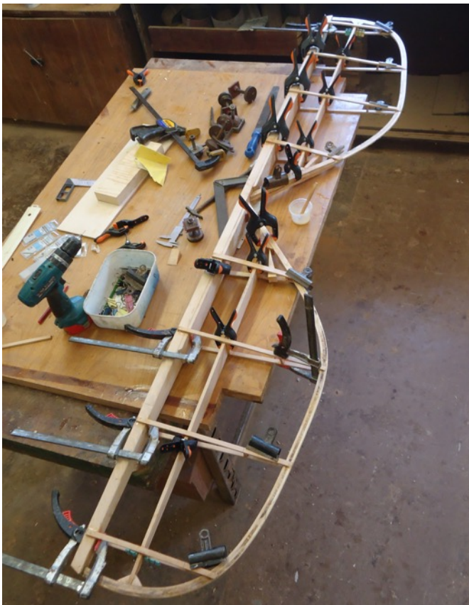
The elevator of John's replica under construction.
