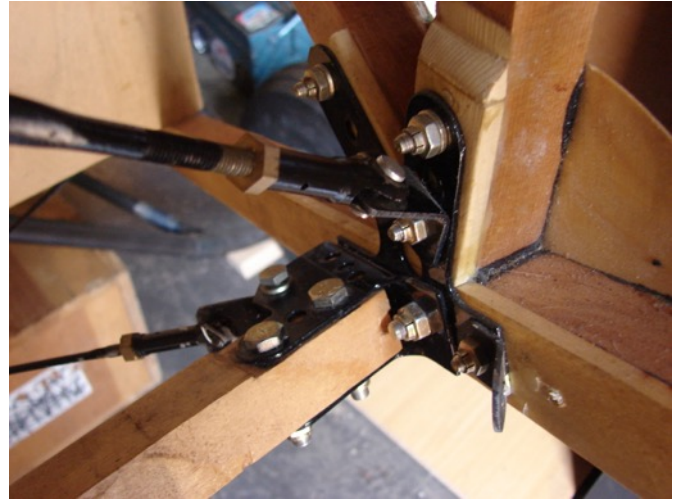
Detail of a typical junction point in the fuselage frame: layers of brackets fulfilling a variety of purposes.
