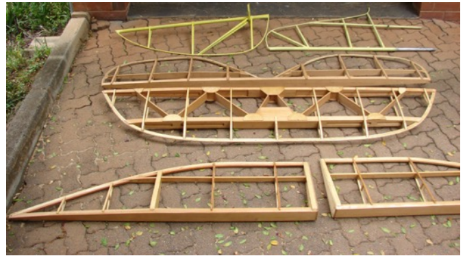
The sub-assemblies that were initially completed: fin and rudder; tailplane and elevator and ailerons.
