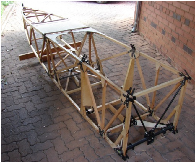
The middle and rear fuselage frames during a trial fitting.
