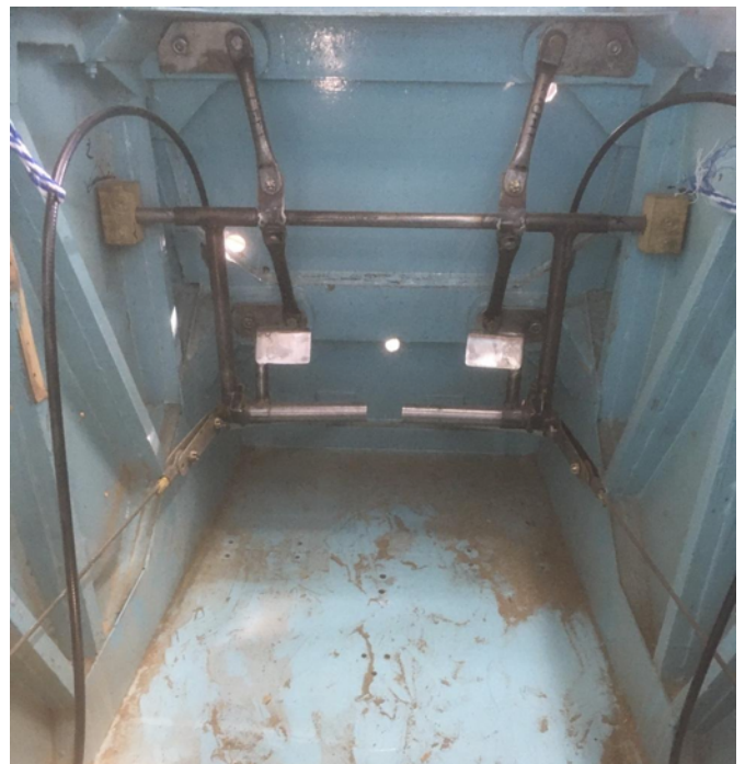
ZS UHG modified with toe brakes
