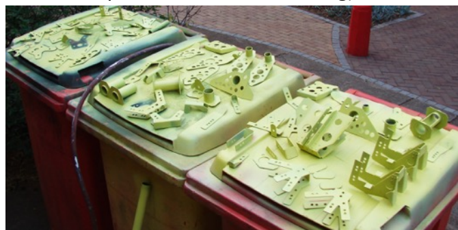
Some of the hundreds of metal fittings being primed with zinc chromate.
