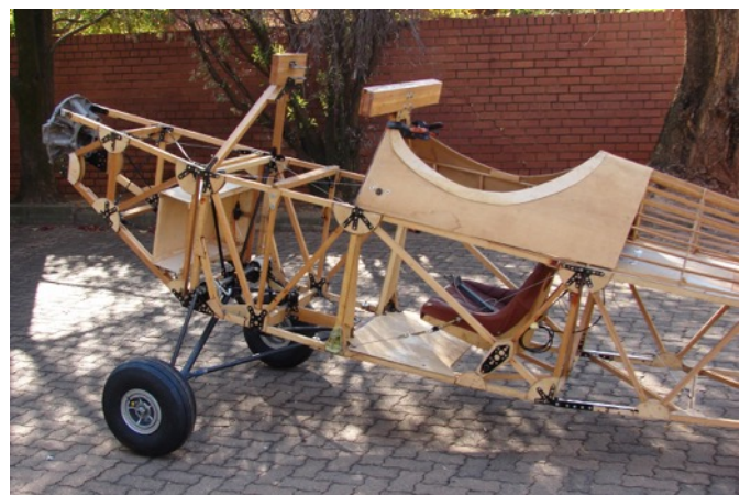
The forward and middle fuselage showing the many metal brackets and the internal bracing.
