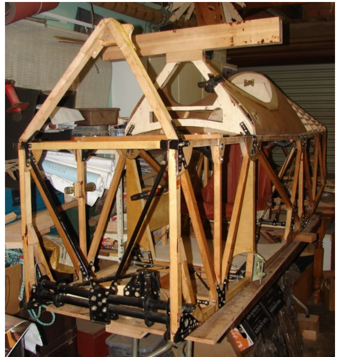
The centre section starts to take shape as part of the middle fuselage. The undercarriage attachments points and the suspension system are also evident.
